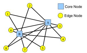
Figure 1. Overlaid star topology that characterises an Agile All-Photonic Network
